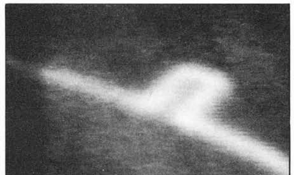
Sample thermograms from an aerial thermography steam distribution system inspection showing a steam leak beneath a street (left). Right thermogram shows the normal thermal expression of an expansion loop.
